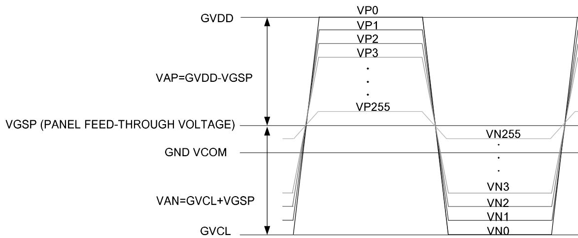
Note: The IC source support maximum LC driving voltage  $VAP$  ( $VAN$ ): 5.224V [  $(GVDD - VGSP) = (VGSP - GVCL) = (GVDD - GVCL) / 2$  ].
