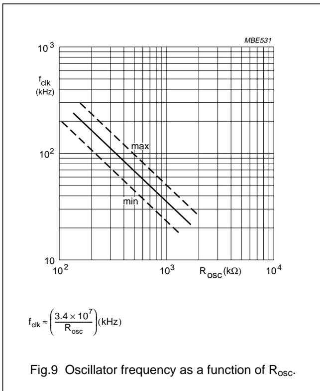
Fig.9 Oscillator frequency as a function of R<sub>osc</sub>.
