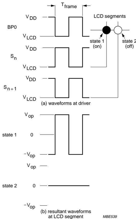
$$V_{state1}(t) = V_{S_n}(t) - V_{BP0}(t)$$
