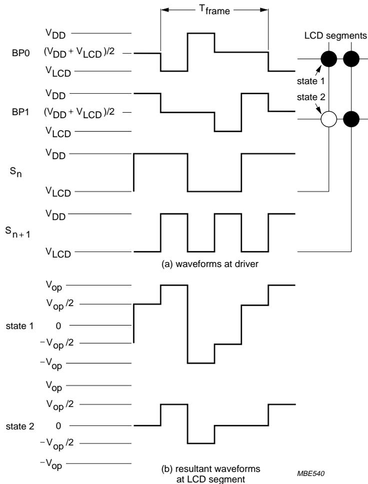
$$V_{state1}(t) = V_{S_n}(t) - V_{BP0}(t)$$
