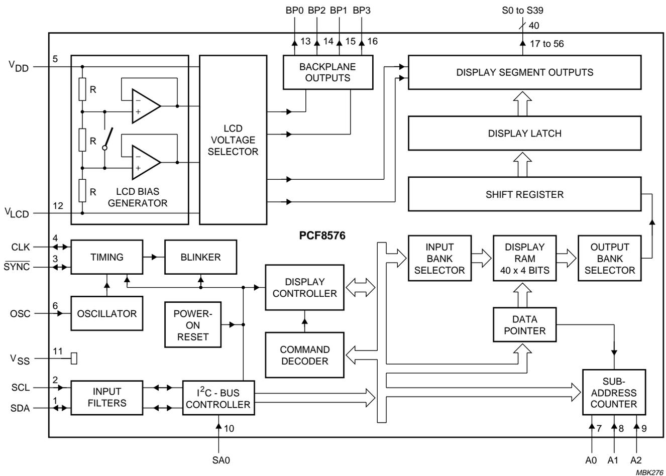
Fig.1 Block diagram (for VSO56 package; SOT190-1).
