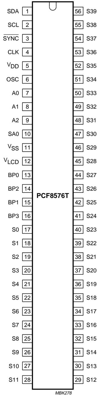
Fig.2 Pin configuration; SOT190-1.
