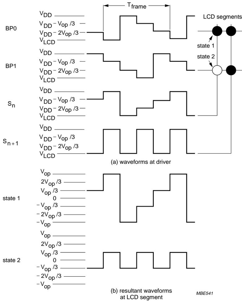
$$V_{state1}(t) = V_{S_n}(t) - V_{BP0}(t)$$
