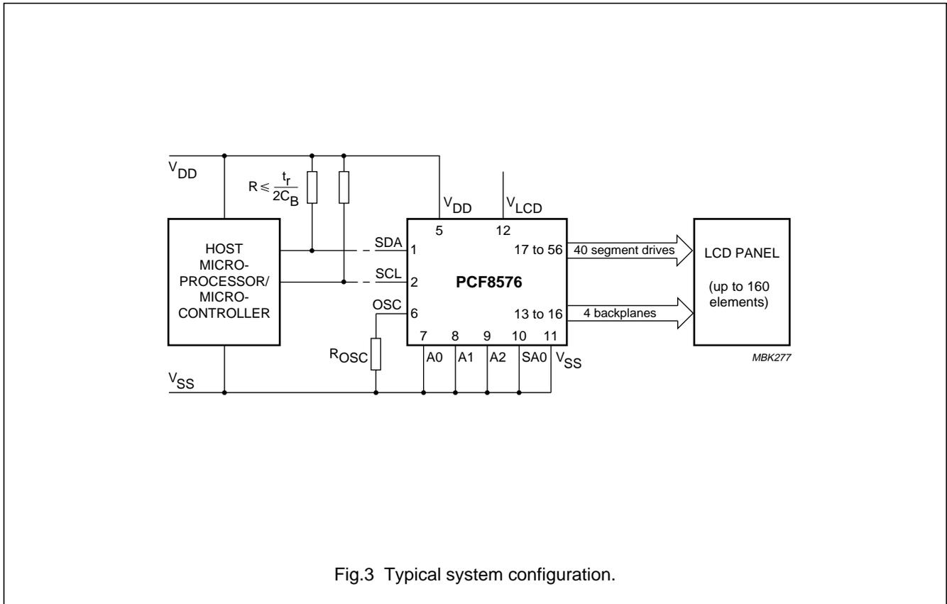
Fig.3 Typical system configuration.
