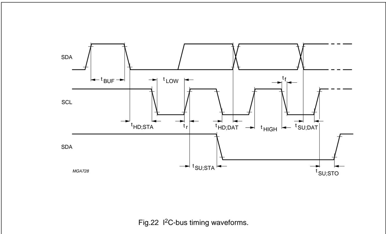
Fig.22 I<sup>2</sup>C-bus timing waveforms.
