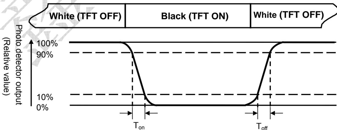
Fig. 10-2 Definition of response time Note 4: Definition of contrast ratio
