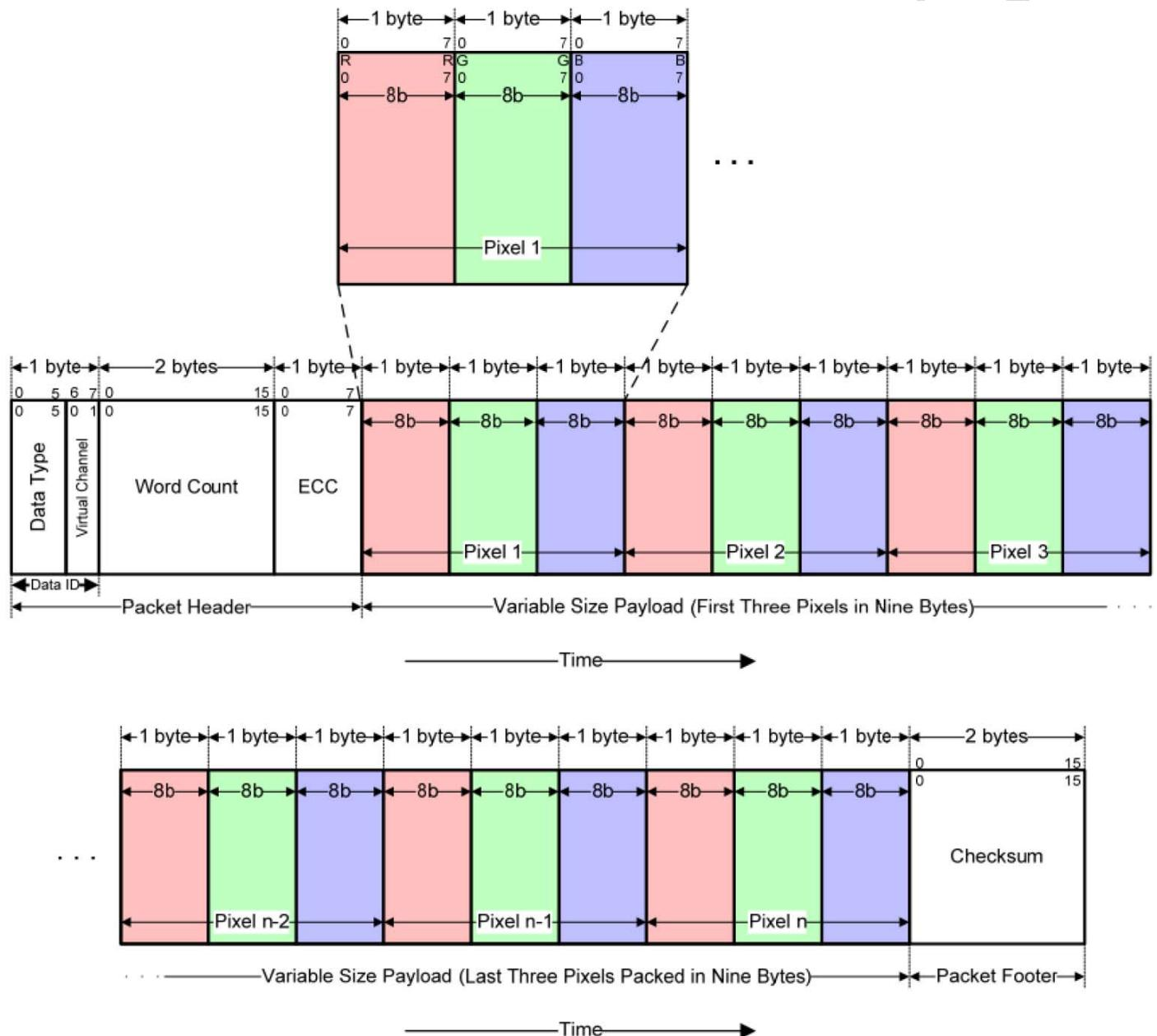
Figure 6-1 DSI RGB888 (24bpp) Color format, Long Packet
